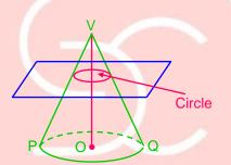
Section of a right circular cone cut by a plane, which is parallel to a generator of the cone is a parabola.
