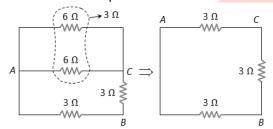
So the equivalent resistance between points A and B is equal to
