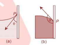
For example when glass strip is dipped in water and mercury as shown in figure (a) and (b) respectively, the angle  $\theta$  is angle of contact, which is acute in case of water and obtuse in case of mercury.
