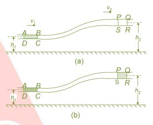
The pipe line is horizontal at *A* and *P* and are at heights  $h_1$  and  $h_2$  respectively from a reference plane. The pipe line gradually widens from left to right. Let  $P_1$ ,  $A_1$ ,  $v_1$  and  $P_2$ ,  $A_2$ ,  $v_2$  be the pressures, areas of cross-section and velocities at *A* and *P* respectively.
