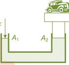
The ratio  $\frac{A_1}{A_2}$  is smaller than 1 and thus applied force can be much smaller than the weight Mg that is lifted.
