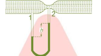
If  $P_1$  is the pressure at point 1 and  $P_2$  the pressure at point 2 we have  $\frac{P_1}{\rho} + \frac{1}{2}v_1^2 = \frac{P_2}{\rho} + \frac{1}{2}v_2^2 \text{ where } v_1 \text{ and } v_2 \text{ are the velocities at these points respectively.}$ We have  $Av_1 = av_2$
