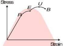
That is on the removal of force body remains deformed. If deformation is further increased, the wire breaks at point *B* called as breaking point. The stress corresponding to this point is called as breaking stress. Before reaching breaking point the curve has a point where tangent to this curve has zero slope. This point corresponds to maximum stress that the body can sustain. This point is called as ultimate point and stress at this point is called as ultimate strength of wire.
